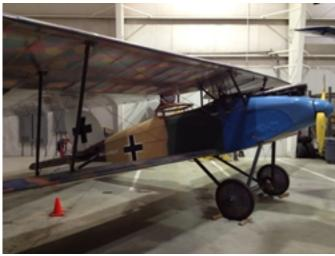
The CL.II is a single engine biplane, with an all wooden structure. The fuselage is covered with thin plywood paneling and houses the crew of two in a single cockpit. It is armed with two fixed 7.92 mm (.312 in) machine guns for the pilot and a flexible 7.92 mm (.312 in) machine gun mounted on a raised ring mount, operated by a rear gunner.
